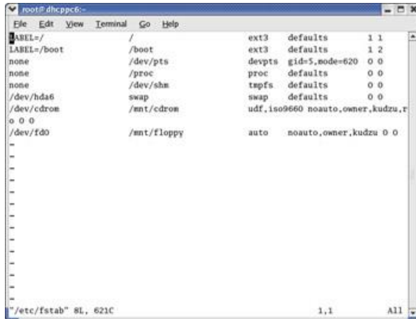
Figure 11-1: A File Displayed in a Full-Screen Text Window by the vi Editor.
